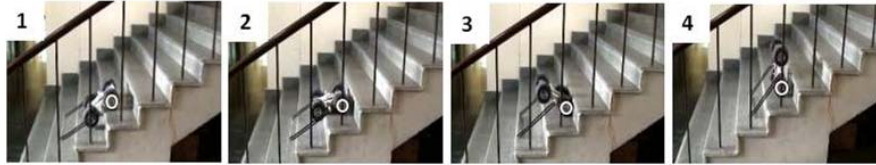
Boombot climbing step with wheel supporting higher weight (marked white) in front
