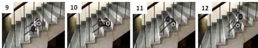
Boombot climbing next step with wheel supporting higher weight having come to the front
