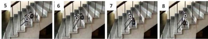
Boombot slipping over step with wheel supporting lower weight in front
