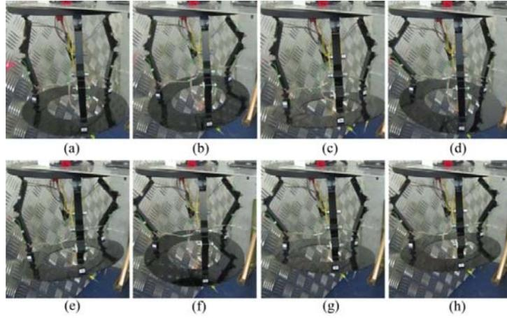
Figure 6: Snapshots of eight binary configurations of the tested prototype of BAPAMAN1: a-OP0; b-OP1; c-OP2; d-OP3; e-OP4; f-OP5; g-OP6; h-OP7.
