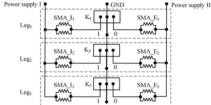
Figure 5: Scheme of the actuator wiring.
