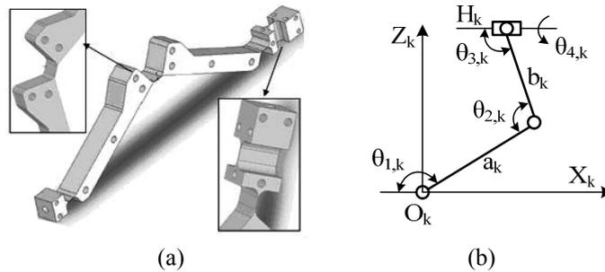
Figure 2: One leg of BAPAMAN1: (a) CAD design; (b) kinematic scheme.
