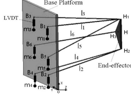
Figure 3: 3D scheme of Milli-CaTraSys with the reference frame O-XYZ
