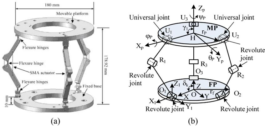
Figure 1: The proposed design of BAPAMAN1: (a) CAD design with main dimensions; (b) kinematic scheme.
