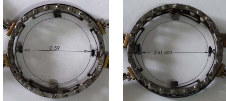
Figure 10: Ring-actuator under testing: (a) before actuation (b) after actuation that resulted in 3 mm increase in the diameter of the circles passing through the clamping pads.
