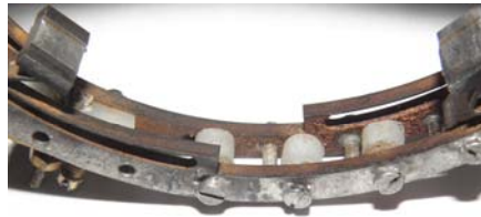
Figure 6: Electrical insulation of the actuator using acrylic roller guides shown with a close-up view of the fabricated ring-actuator.
