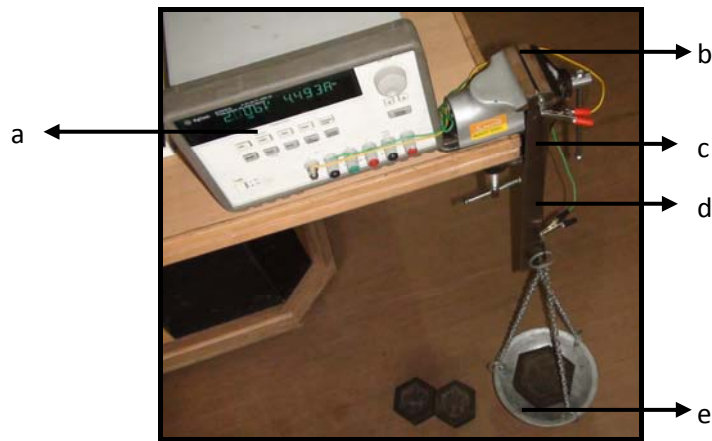
Figure 3: Experimental setup for calculating the stiffness of the SMA wire in martensite and cooling phases. (a) Power supply (b) Bench Vice (c) Ruler (d) SMA wire (e) Weight
