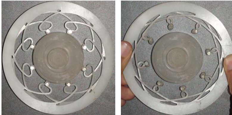
Figure 1: Circumferentially-actuated radially deployable compliant mechanism prototype (a) deformed and grasping a circular object (b) undeformed with the release of the grasp.
