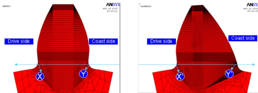
Figure 9a: Schematic of symmetric gear root section
