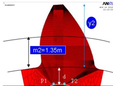
Figure 4b: Schematic of .35m dedendum gear
