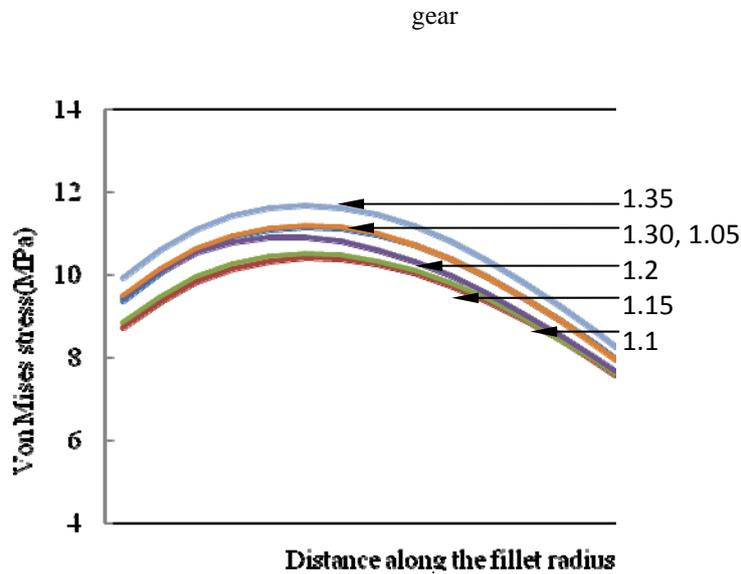
Figure 3: Induced stress at drive side fillet profile
