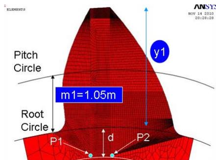
Figure 4a Schematic of 1.05m dedendum gear
