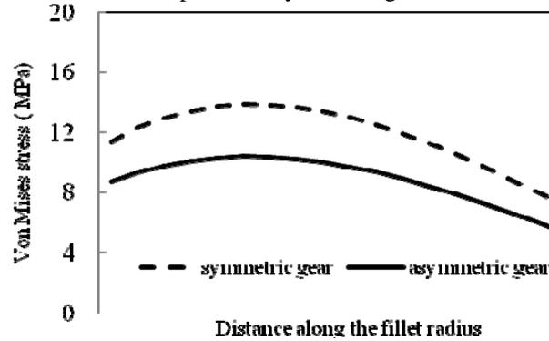
Figure 7: Drive side stress: Symmetric and asymmetric
