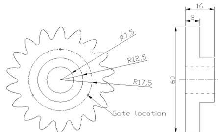
Figure 1b: Detailed of chosen asymmetric gear
