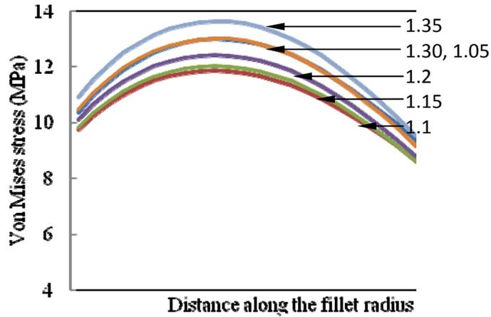
Figure 5: Coast side fillet profile for the different designs
