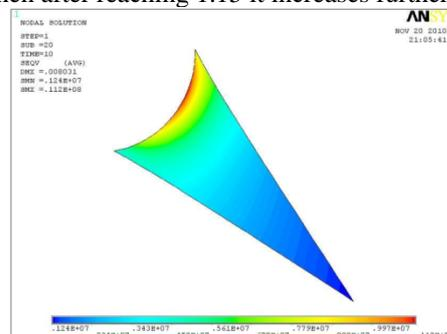
Figure 2b: Identification of maximum stress along the fillet Stress at 1.05m dedendum
