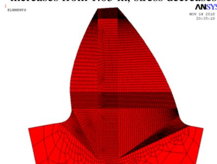
Figure 2a: Finite element model of single gear tooth
