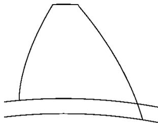
Figure 1a: Different base circle diameter of drive and coast side of asymmetric gear tooth
