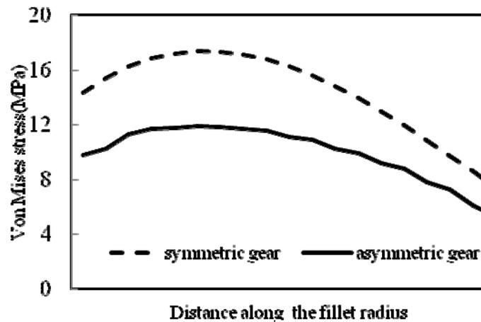
Figure 8: Coast side stress- symmetric and asymmetric
