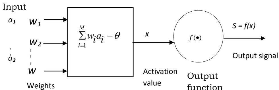
Fig.2 A typical neuron model
