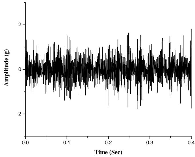
Fig. 3. Typical unbalance time domain vibration acceleration plot
