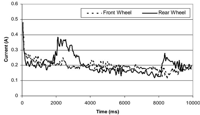
Figure 3.5: Motor current variation in front/ rear motor (front wheel climbs the step)
