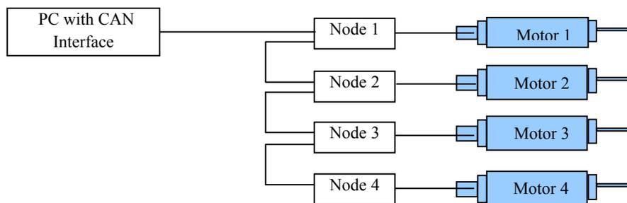
Figure 3.1: Connection diagram of rover with wheel motors
