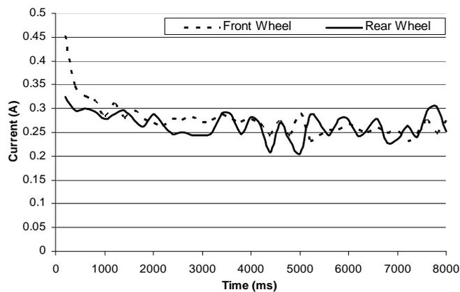
Figure 3.4: Motor current variation for the front & rear motor on an inclined surface
