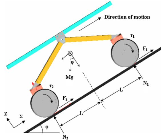
Figure 2.2: Rover traversing up an inclined terrain
