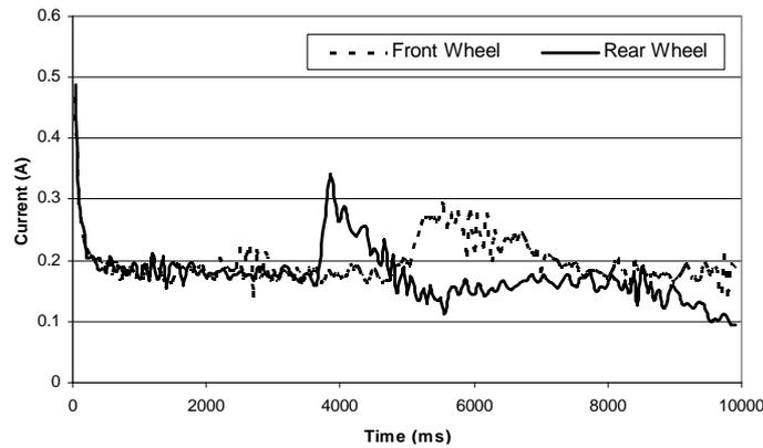
Figure 3.6: Motor current variation in front/rear motor (rear wheel climbs the step)
