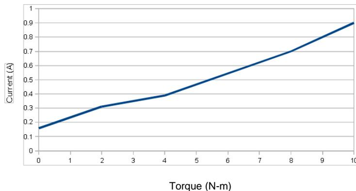
Figure 3.2: Motor Torque-current characteristics for 24V input
