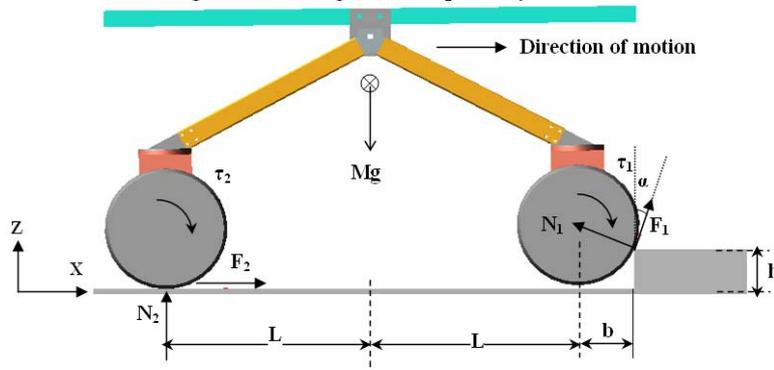
Figure 2.3: Rover climbing a small step (front wheel over step)
