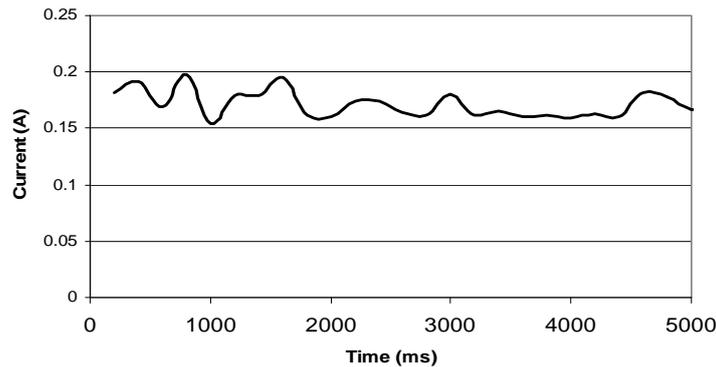
Figure 3.3: Motor current variation on a flat surface
