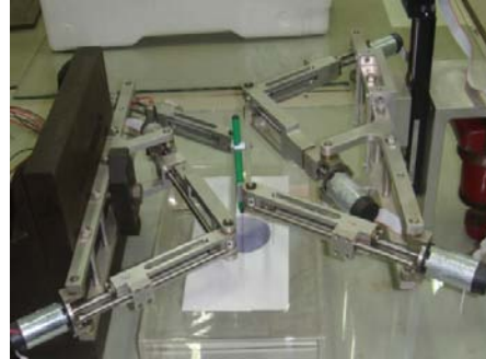
Figure 10: Planar Parallel Robots performing a Common Task in cooperation
