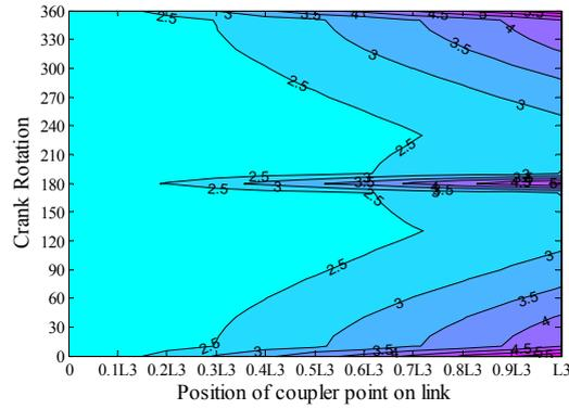
Figure 7: Error zones for mechanism operation.
