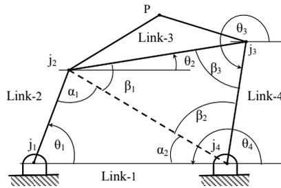
Figure 2: Four Bar RRRR mechanism
