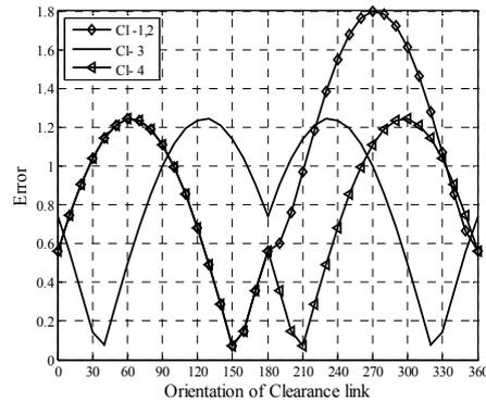
Figure 4: Effect of clearance individual link on error
