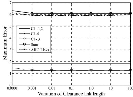
Figure 9: Effect of Clearance link length variation on Error
