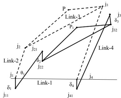
Figure 3: Shift in coupler position due to clearance link
