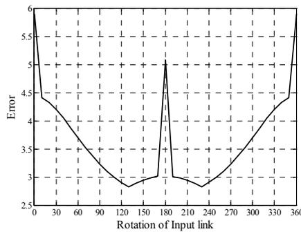
Figure 6: Variation of error for crank rotation
